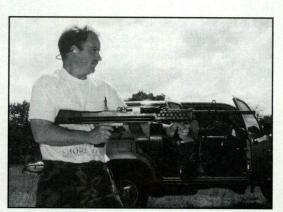
Firing the CMG-2 to judge muzzle rise. There is virtually none, because the bolt "runs out" its travel on the recoil-no jarring stop.
