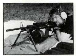
Colt's CMG-2 fed smoothly and had little recoil. It stayed remarkably well on target. Having the cocking mechanism be the rear pistol grip was kind of awkward at first, but once the gunners got used to it, this system had its advantages. You didn't have to break your trigger grip or line-of-sight in order to cock the bolt.
