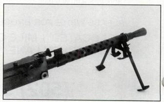
This air-cooled Browning .30 caliber M1919A6 and the A4 series just use a protective sleeve with holes to shield and protect the moving barrel. The holes again assist in air circulation around the barrel and prevent heat buildup.
