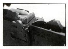
This close-up view of the inside of the receiver shows the large bolt catch being lifted into position by the magazine follower. The hammer, trigger and other fire-control components are mechanically interchangeable with the 5.56 mm semi-auto variants.
