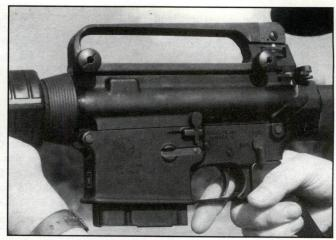
This view of the left side of the new ArmaLite AR-10A4 shows the large knobs on the quick-detachable rear sight/carrying handle assembly. The magazine pictured is the 10-round capacity magazine furnished with the weapon.
