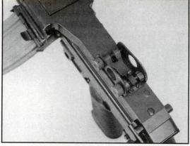
Rear sight of the new style M249 with the 30-round M16 magazine inserted.
