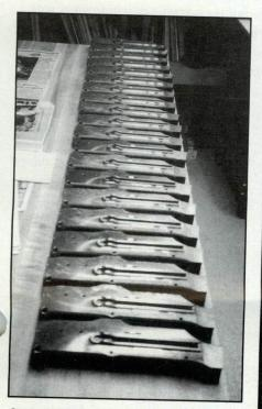
Completed receivers on the bench after final inspection.
